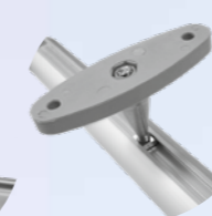
6 Anchoring on profile rail: possible along the whole length by means of square nut; for adjustable ceiling mount RVS/DS or with ceiling bracket RVS/DH. Max. spacing: 2 m.
